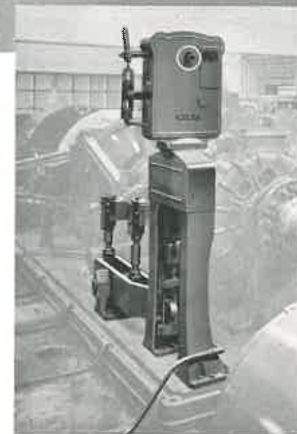
Dynamometer Weightograph for Testing Motors.
